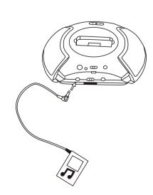
(7) other audio device can be connected with portable speaker system by stereo cable insert to the socket "input"
